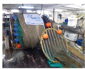
The Flexgrid during fshing operations and detail of a rigid TED used in sea trials.
